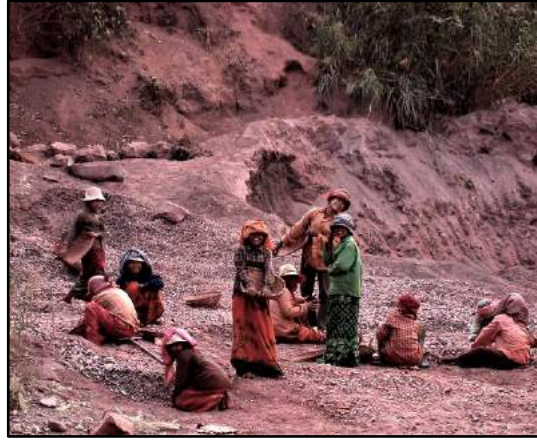
Labour based aggregate production Photo J Cook
