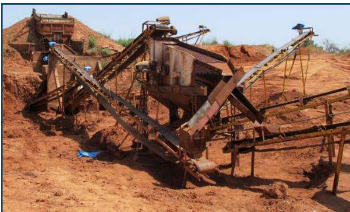
Medium sized crushing and screening plant used for a LVR network rehabilitation Photo J Cook
