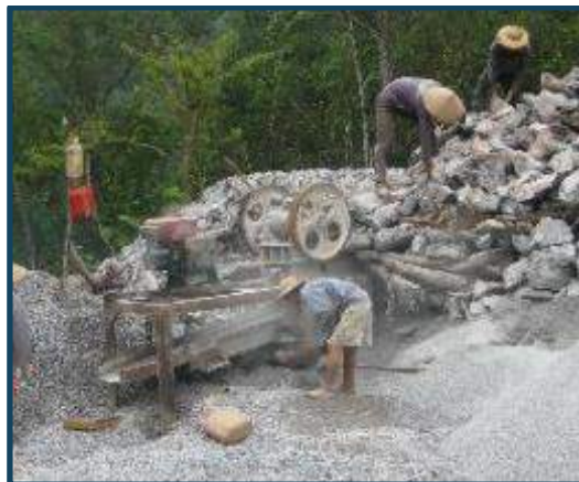
Small mobile crusher combined with screen Photo J Cook
