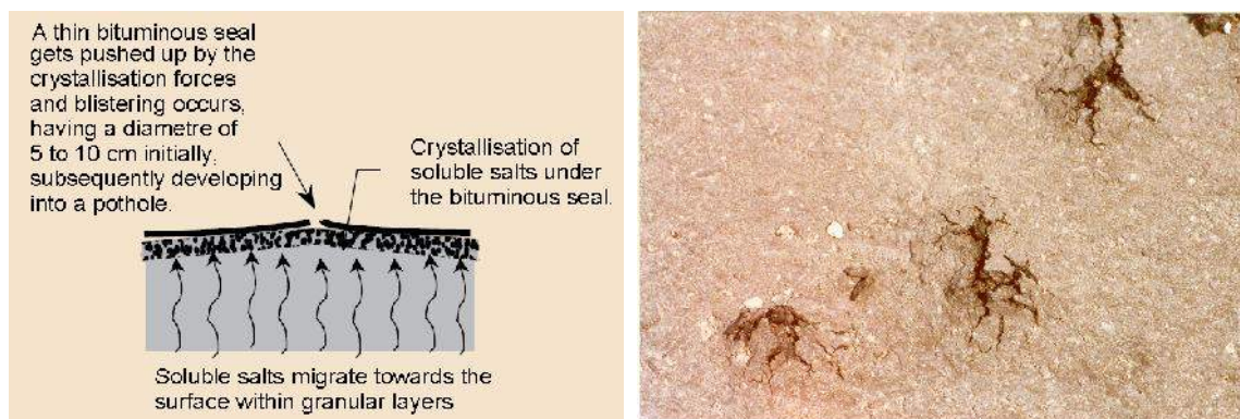
Figure 4-14: Mechanism of salt damage
