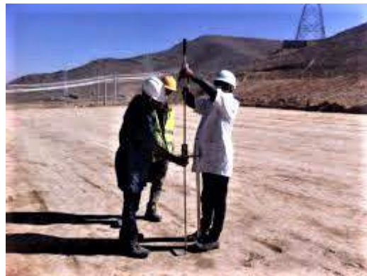
Figure 4-1: Team of three persons required for DCP testing
