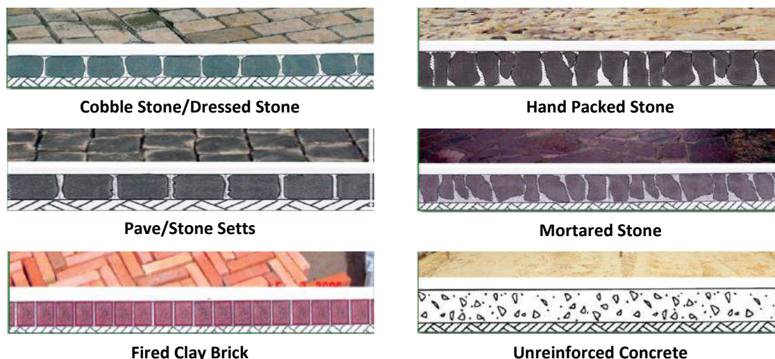
Figure 12-9: Common types of non-bituminous surfacings
