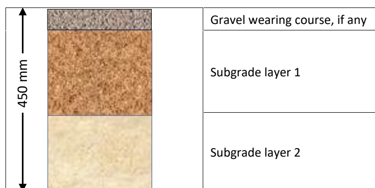
Figure 4-3: Typical soil profile in test pit
