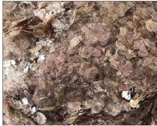
Figure 4-17: Micaceous soil with large flakes of muscovite
