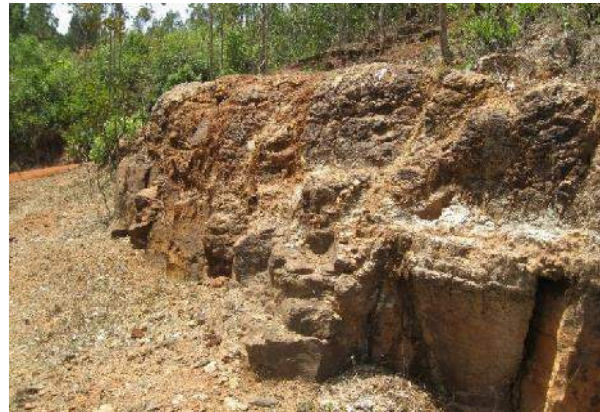
Figure 4-22: Variable degrees of weathering in quarry
