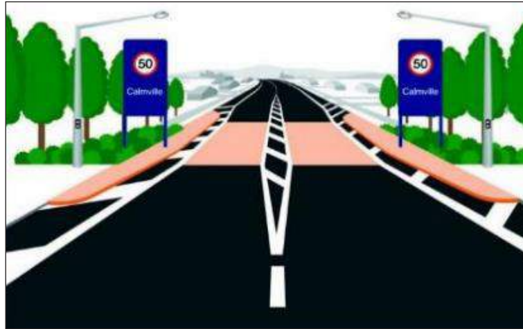
Figure A.7.8: Road narrowing
