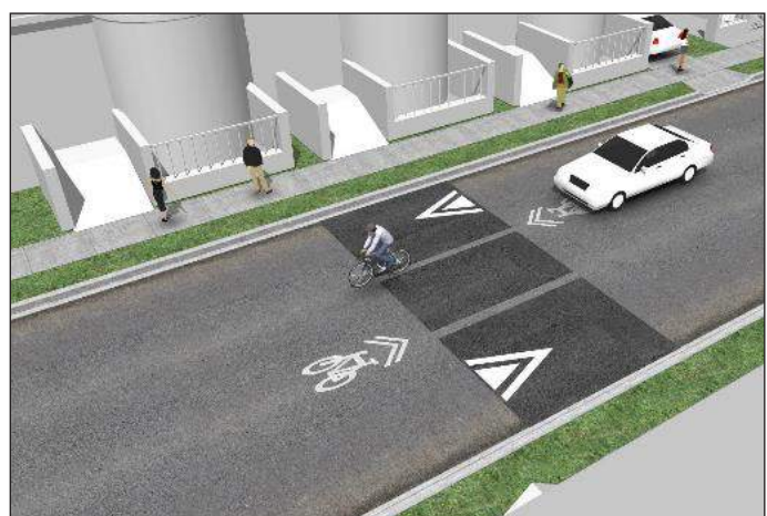
Figure A.7.5: Speed cushion application
