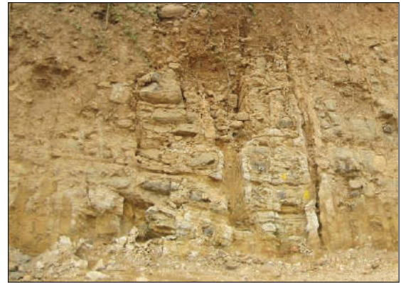
Weathering grade changes laterally as well as with depth (WG decreases in direction of arrows). Note the infilled vertical joints.
