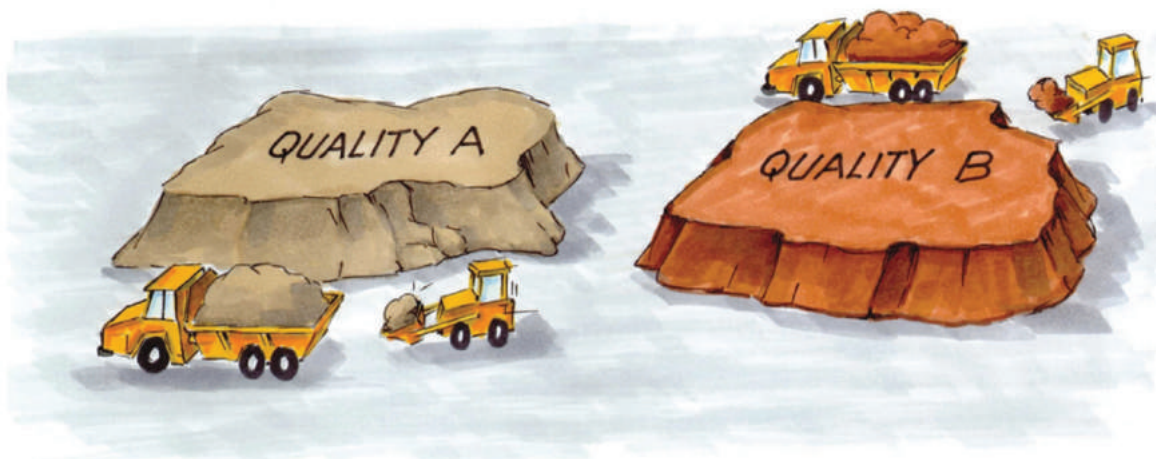
Figure B.10.13: Loading from two separate stockpiles in the borrow pit
