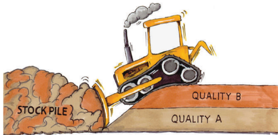
Figure B.10.12: Unrecommended method for blending in borrow pit
