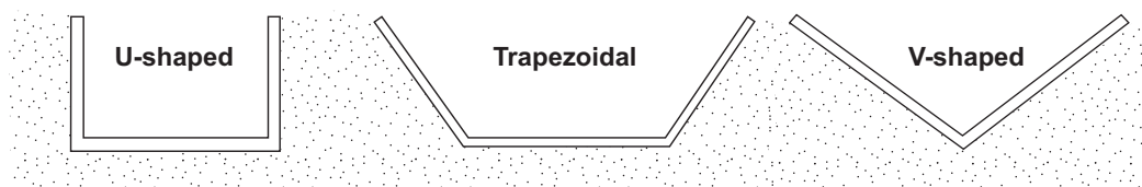
Figure C.4.1: Typical side drain cross-sections
