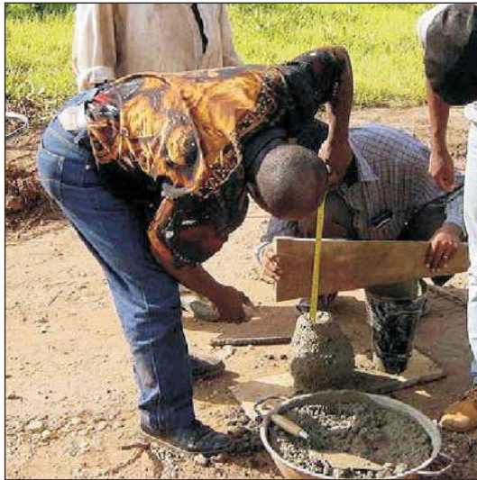
Figure C.8.10: Workable and cohesive concrete Figure C.8.11: Collapsed slump - too much water
