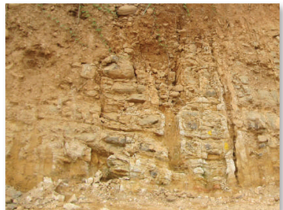
Weathering grade changes laterally as well as with depth (WG decreases in direction of arrows). Note the infilled vertical joints
