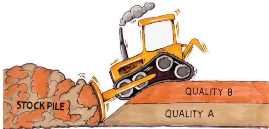
Figure B.10.12 Non-recommended method for blending in borrow pit
