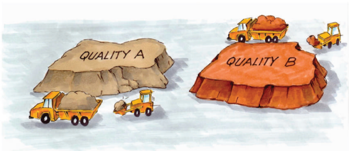
Figure B.10.13 Loading from two separate stockpiles in the borrow pit
