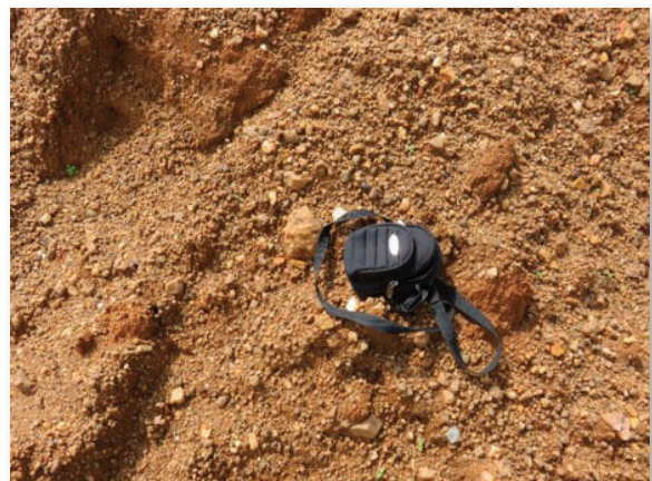
Figure B.10.2 Typical lateritic and quartzite gravels found at or close to the ground surface
