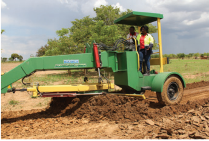
Figure 2. Rogue heavy (5 t) towed grader (Photo: Intech; reproduced with permission of Intech Associates)
