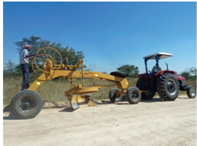
Figure 1. Mann light (2 t) towed grader (Photo: Intech; reproduced with permission of Intech Associates)
