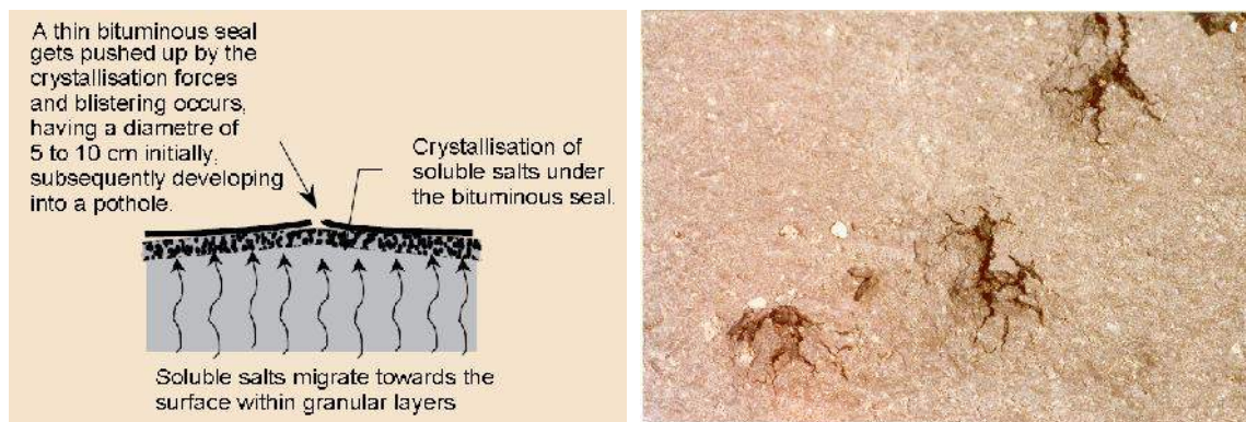
Figure 4-15: Mechanism of salt damage
