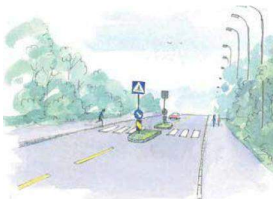
Figure 4-10: Pedestrian crossing with refuge island
