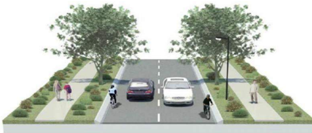
Figure 2-2: Typical idealised layout of a local residential street (Class 5)
