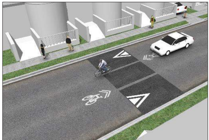
Figure A.7.5: Speed cushion application
