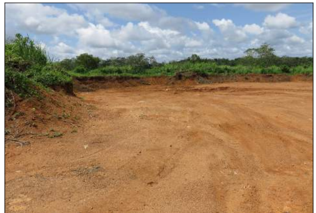
Figure B.10.1: Shallow surface deposit extraction results in high land take : volume ratio
