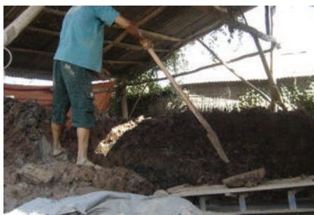
Clay is moved to moulding machine
