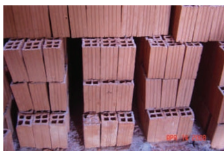
The hot air can blow through all brick rows. (Note that the hollow bricks shown are not suitable for road paving).
