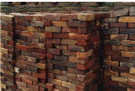
Burnt clay bricks stacked ready for use.
