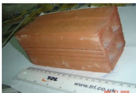
4 void brick (7 x 7 x 16)cm (Note that the voided brick shown is not suitable for road paving).
