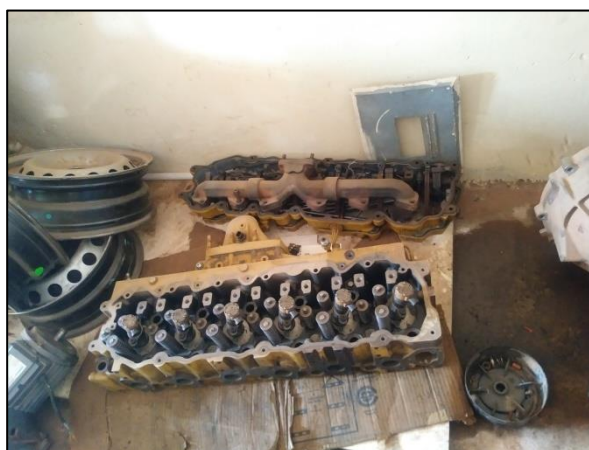
Figures 3 & 4 Cracked cylinder sleeve and defective cylinder head of the Chongwe motorgrader
