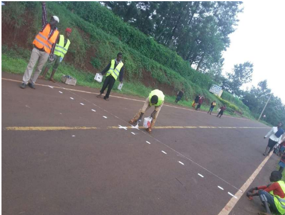
Figure 14: The dashed line marking the boundary of the destructive testing panel of the LTPP section
