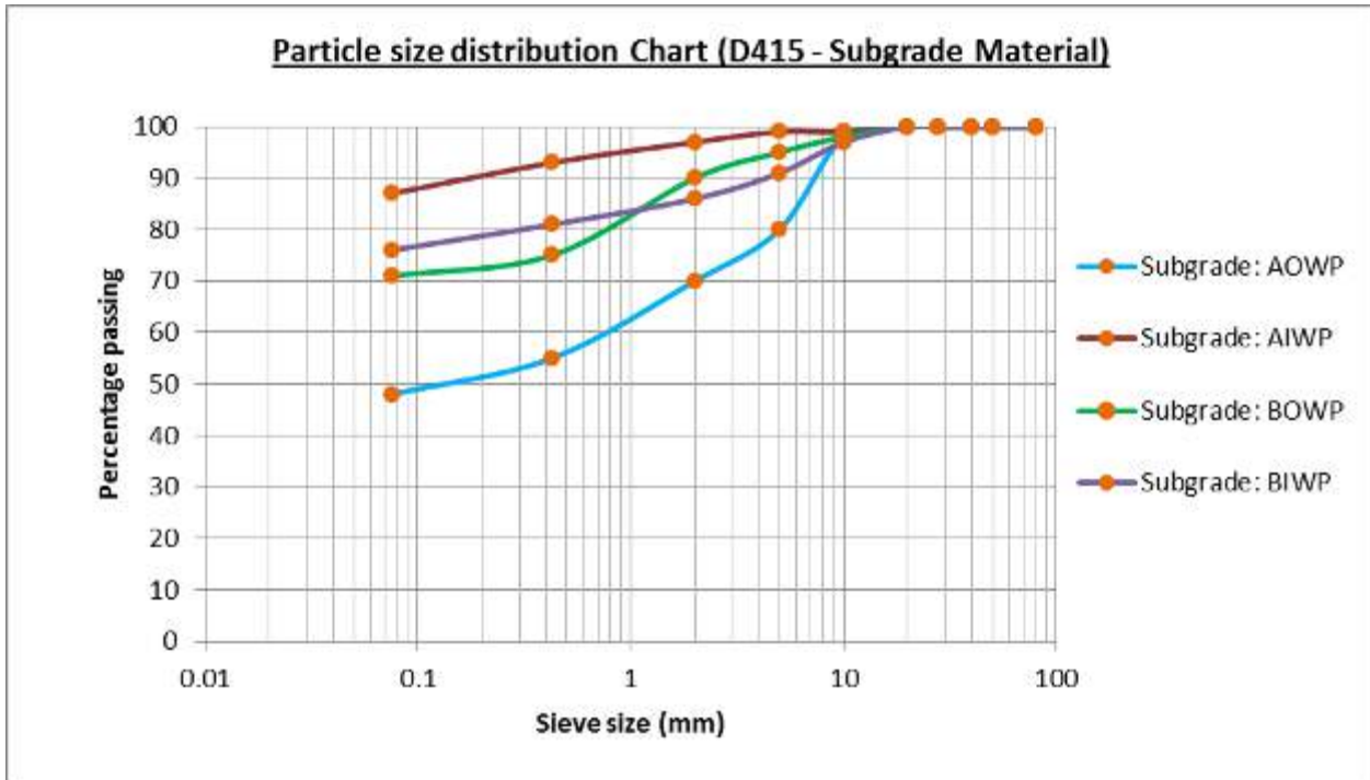
Figure 7-8: Particle size distribution for subgrade material (D415)
