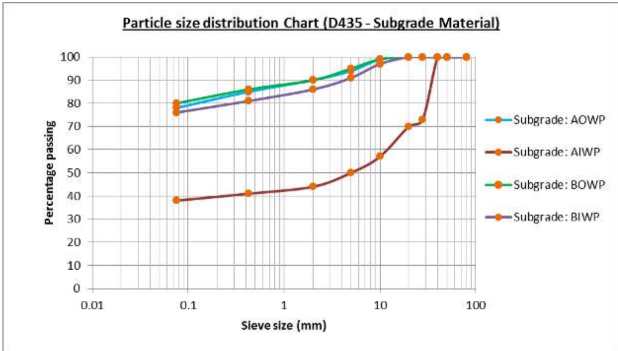
Figure 11-8: Particle size distribution for subgrade material (D435)
