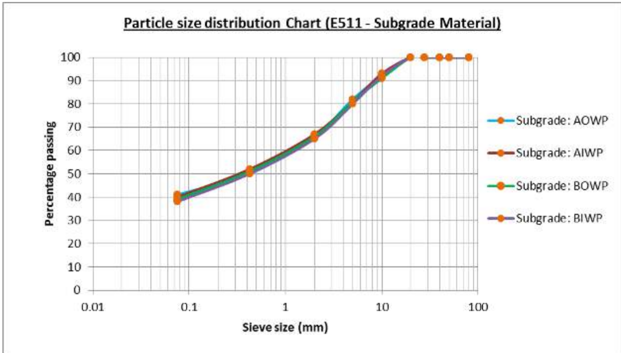
Figure 12-8: Particle size distribution for subgrade material (E511)
