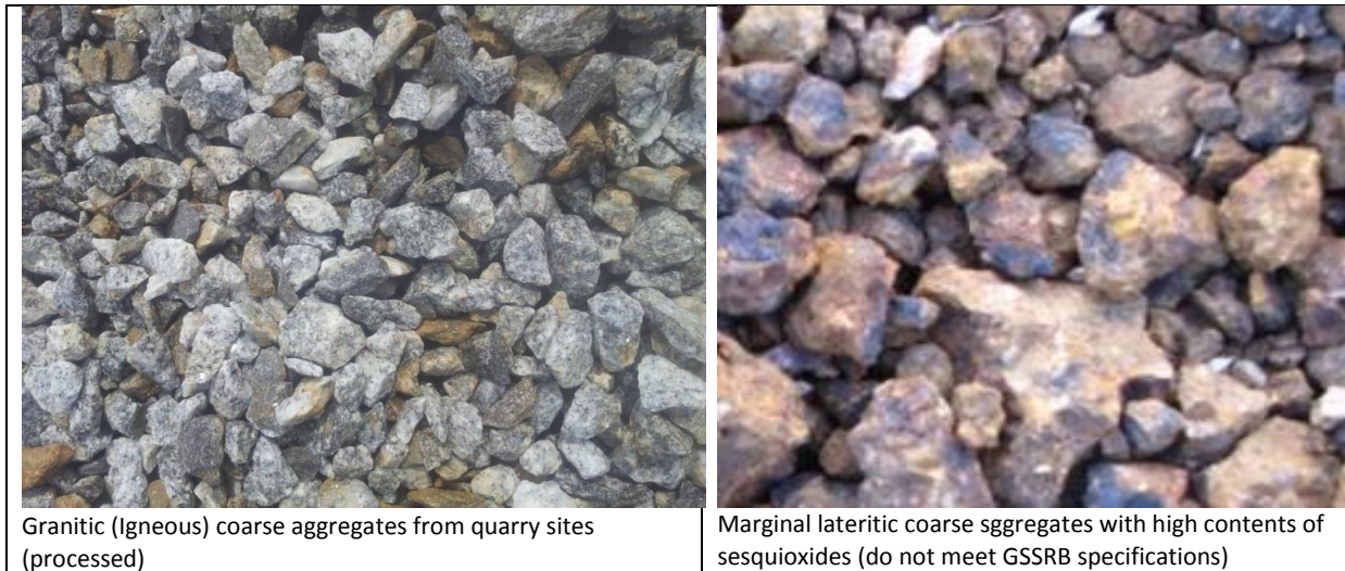
Figure 5-1: Granitic coarse aggregates for road construction in Ghana
