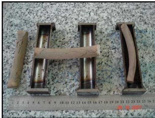
Plate 3. Linear Shrinkage Testing
