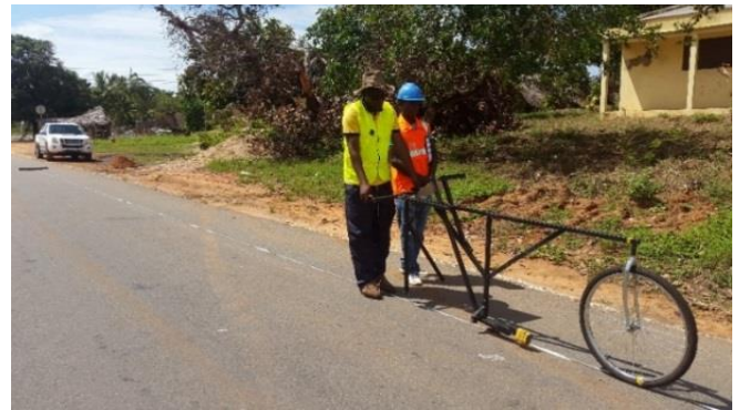
Fig. 4. Illustration of the measurement of Roughness with the MERLIN.
