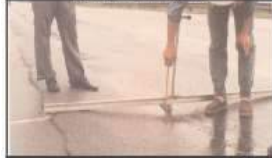
High severity with rut depths > 25 mm
