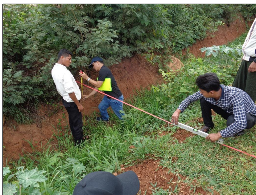
Figure 8: Measuring the Drainage Factor
