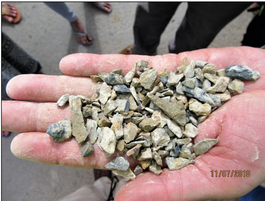
Figure 5: Flaky Aggregate used in DBST
