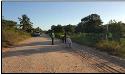
Gravel loss measurement before grader passed on the Control section
