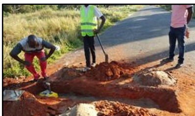
Testing of insitu density and moisture content on all layers on Dabo's section
