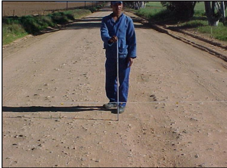
Figure 5: Measuring gravel loss
