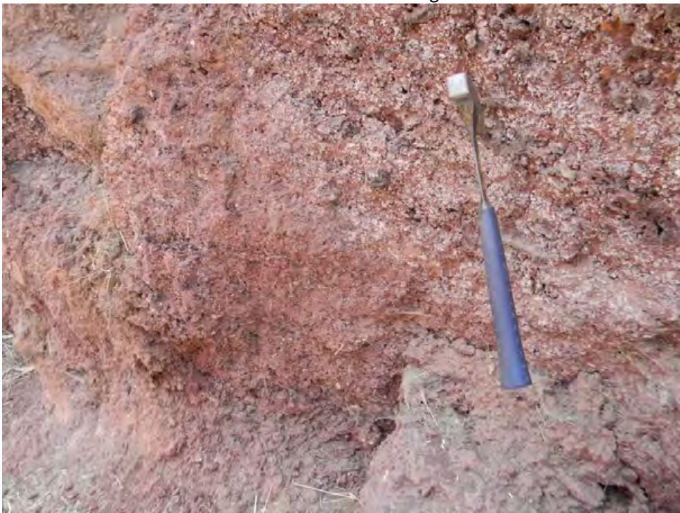
Material 2: stratified, dense, cinder gravel
