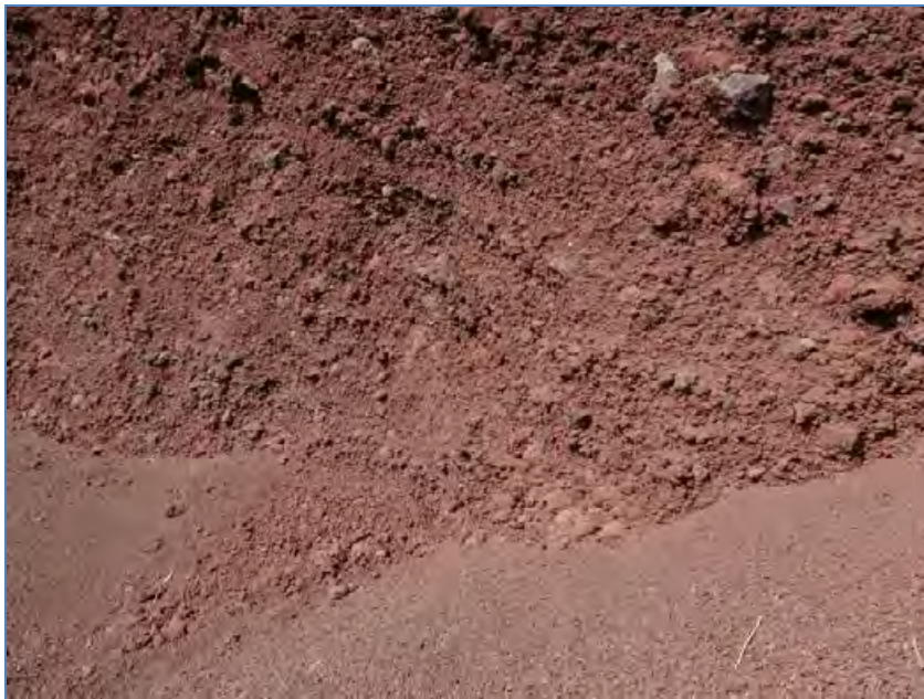
Figure 17: Granular cinder material
