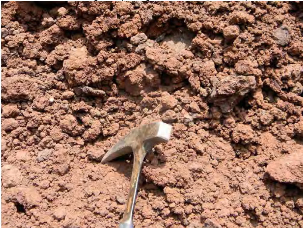
Some fines content can be identified as well as a loose structure
