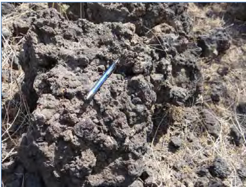
Figure 8: Boulder of very hard grey-black-coloured cinder
