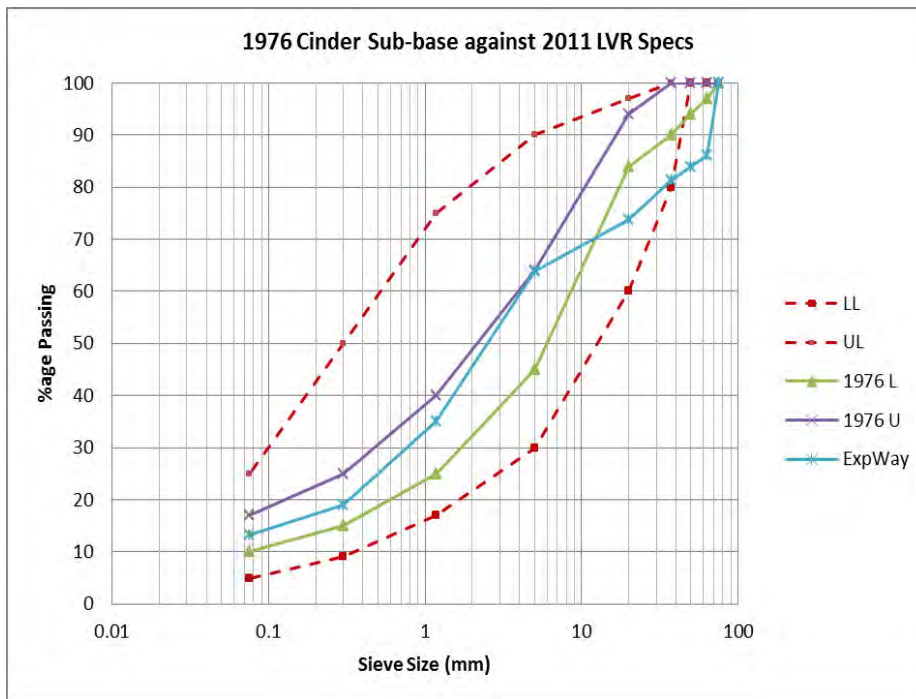
Figure 2: Comparison of 1976 cinder sub-base grading to the ERA 2011 LVR Manual requirements
