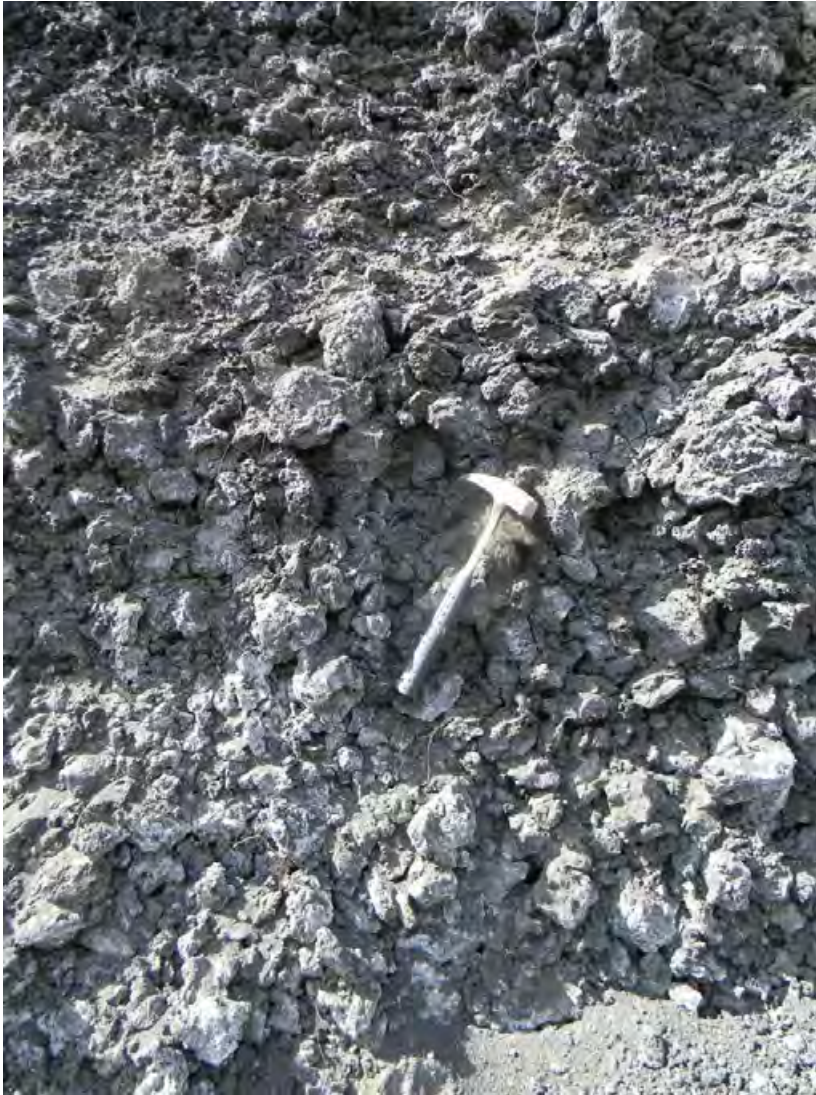
Voided deposit of cinder bombs, fines probably washed out in groundwater
