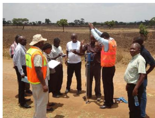
Figure 2: DCP test on S126 Linthipe- Lobi
