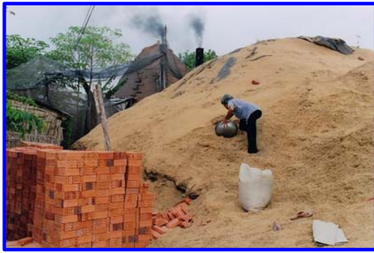
Photos 6 and 7 – Rice husk burnt clay brick production and paving
