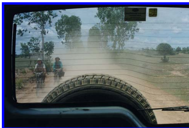
Figure 1 Dust emissions from gravel road in the dry season
