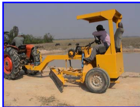
Photos 8 and 9 – DTW designed towed grader for road maintenance
