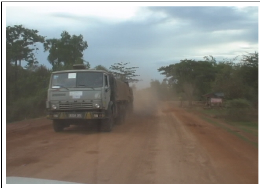
Figure 12 - Dust clouds on gravel roads created by vehicle passage in dry season can adversely affect visibility: drivers would not have a clear view of overtaking vehicles.
