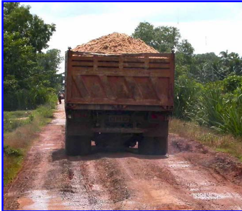
Figure 1.3: Overloaded Truck on the Puok Trial Road (Section 4)
