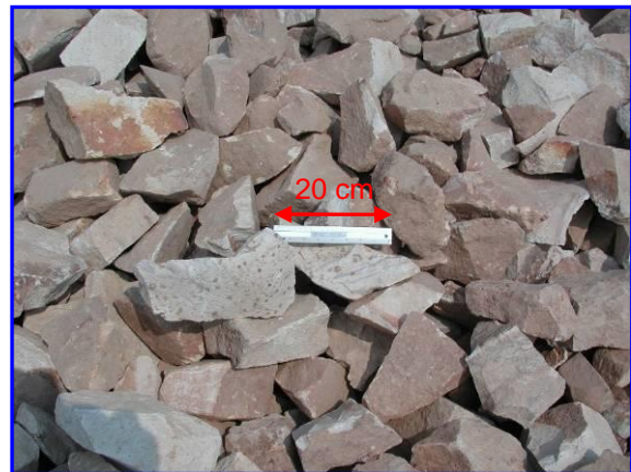
Trials Figure A1-4: Q3-Hand-broken stone aggregate 100 – 200 mm size from Phnom Leap
