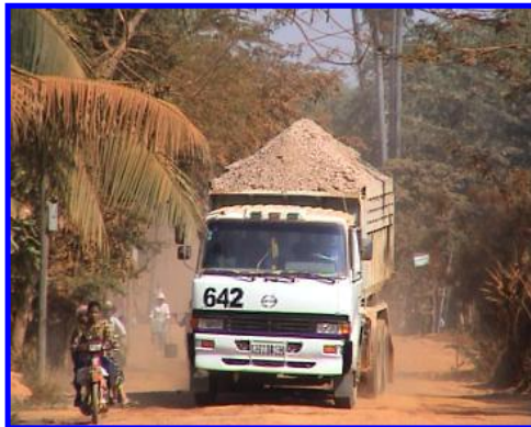
Image 1 – Truck bodies extended in Cambodia to carry at least 20m 3 of construction materials on 3 axles.
