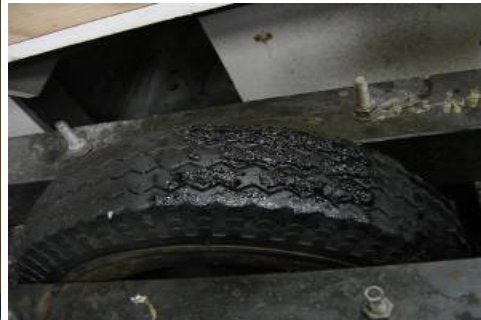
Tyre with bitumen adhered.
