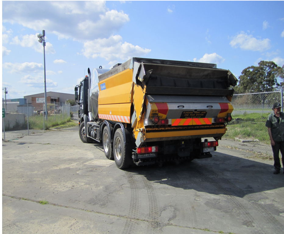
French synchronized spraying / spreading equipment
