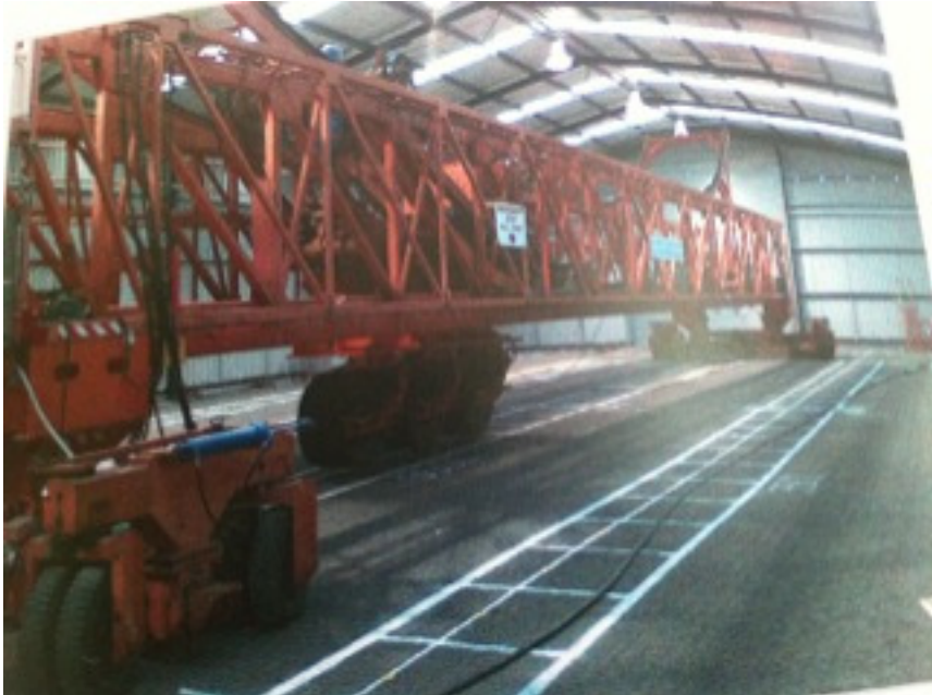
Accelerated Loading Facility (ALF)
