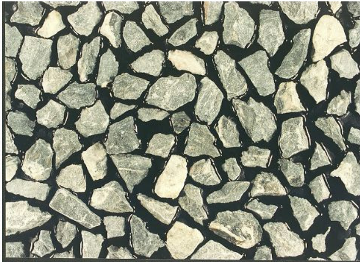
Typical spread of aggregate for a Cape Seal
