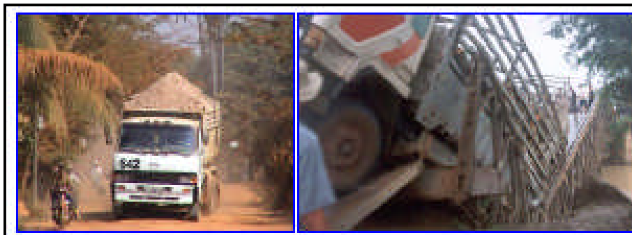
Figure 3.1 Overloading and risk of related structures failure are important considerations for some routes
