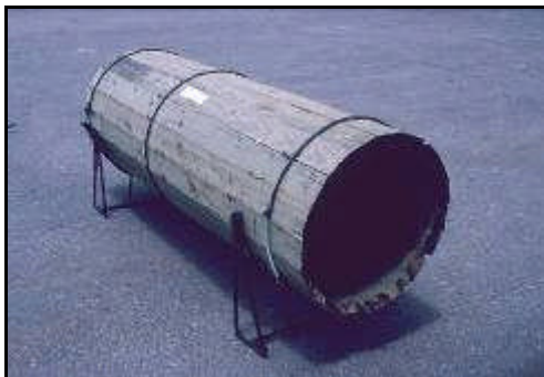
Figure 7.44 Treated timber culvert
