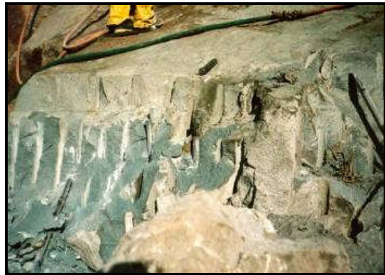
Figure 7.3 Hand quarrying of stone
