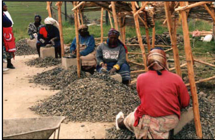
Figure 7.46 Aggregate can be crushed and screened by hand or machine
