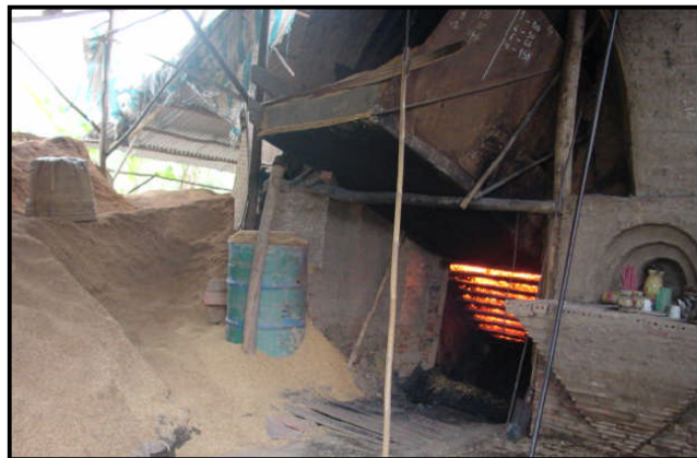
Figure 7.28 High quality burnt clay bricks produced in small 'beehive' kilns fired by rice husk. Bricks can be fired using coal, wood or other agricultural waste products.
