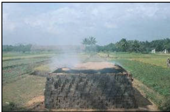
Figure 7.29 Simple burnt clay brick clamp
