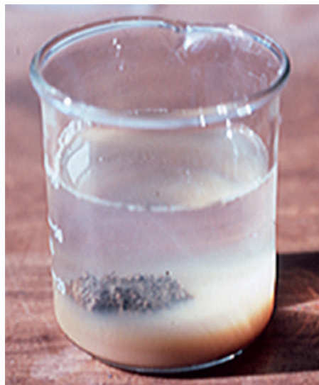
Figure 6-8: Dispersive soil in water (crumb test) showing suspension that does not settle out
