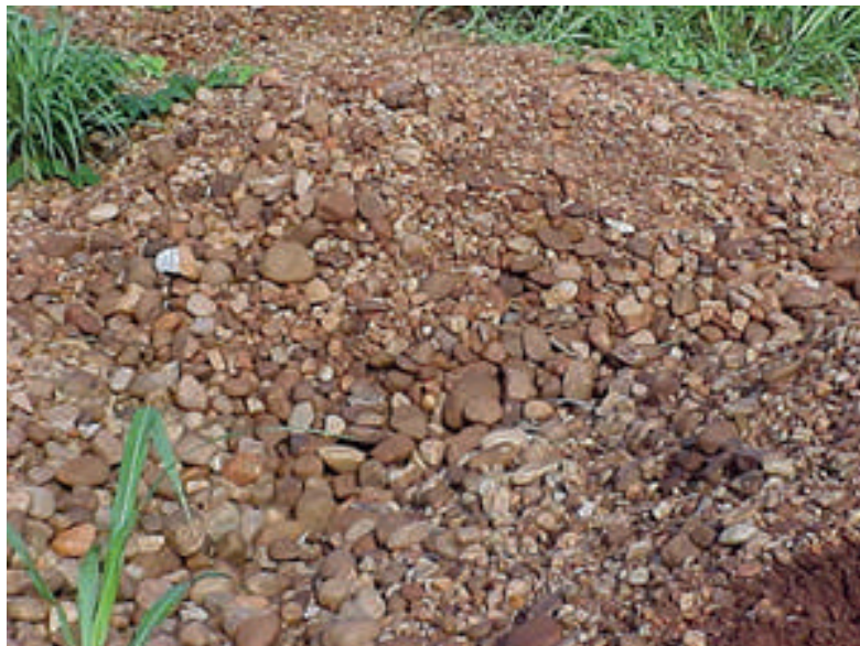
Figure 7-4: Coarse river gravels can be crushed and used for concrete and/or surfacing works
