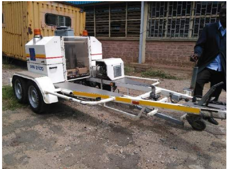
Figure 7 FWD Field Testing Equipment
