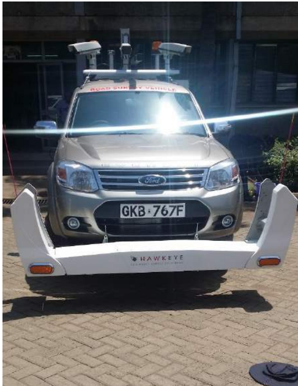
Figure 8 Road Condition Profiler Field Testing Equipment
