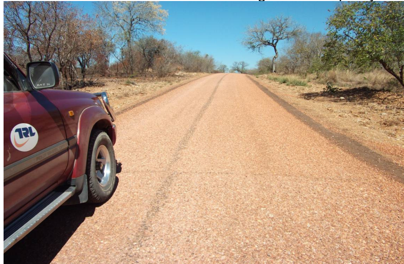
Figure 2: End of section with 1.6L/m 2 binder and beginning of section with 1.4L/m 2
