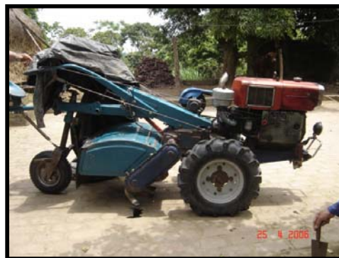
Plate 5 Agricultural rotavator that may be used for mixing lime or cement stabiliser
