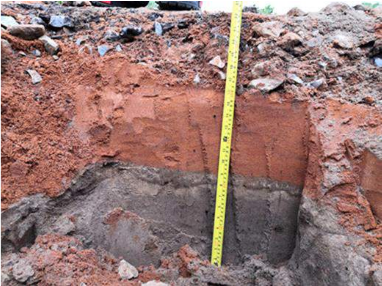
Figure 12 Test pit on Section 1 Macia – Chokwe with probable neat sand sub-base
