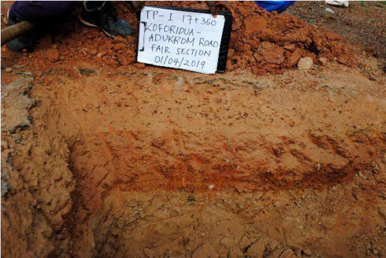
Figure 6 Test Pit on Section 2 Koforidua - Adukrom
