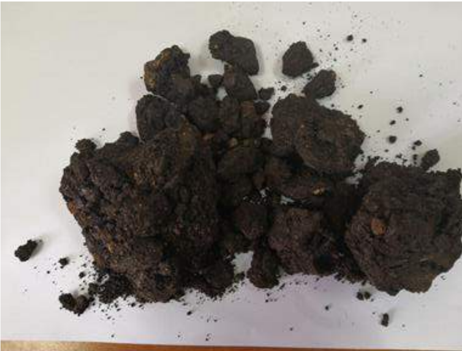
Figure 7 Clayey subgrade (possibly black-cotton soil) observed on Boane – Namaacha Section 1
