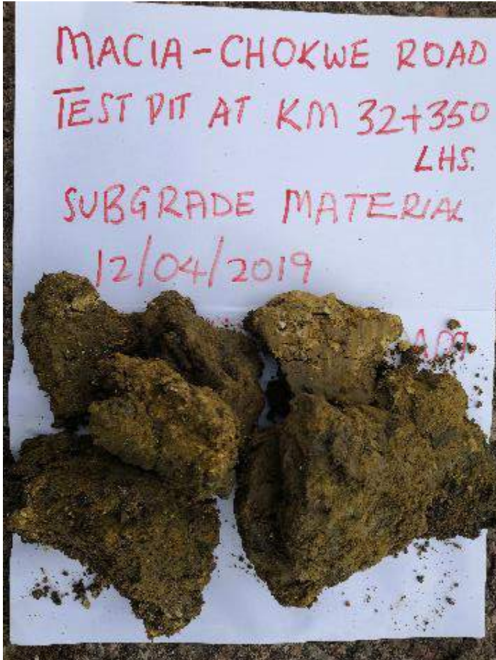
Figure 14 Subgrade on Section 2 Macia - Chokwe
