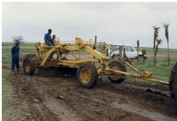
Figure 5.5 – Pre-World War 2 Caterpillar tractor towed grader with rubber tyre modifications. Still in regular use after 50 years (Image: Intech Associates)
