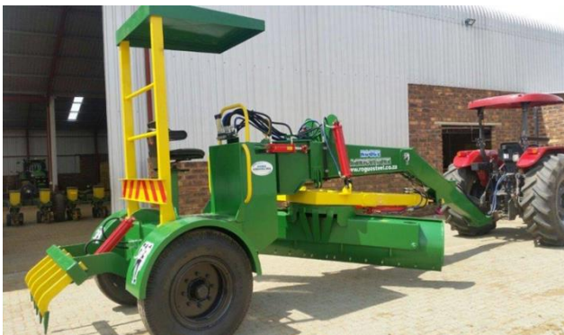
Figure 5.4 – 5 tonne towed grader manufactured in RSA (Image: Intech Associates).
