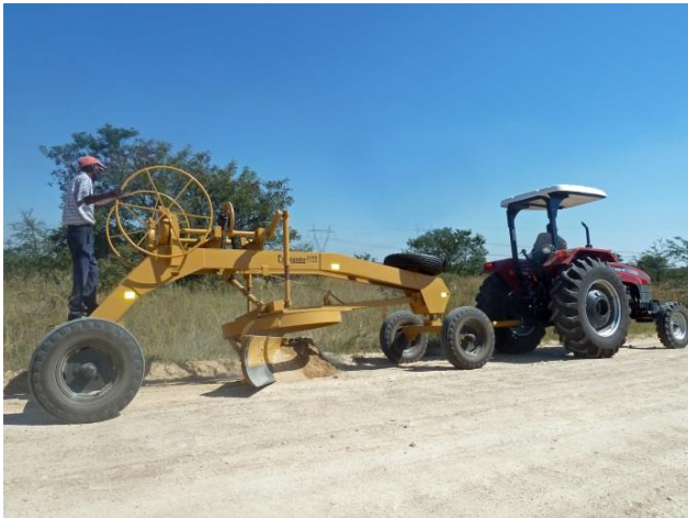
Figure 5.3 – 2 tonne towed grader manufactured in Zimbabwe for more than 50 years (Image: Intech Associates).
