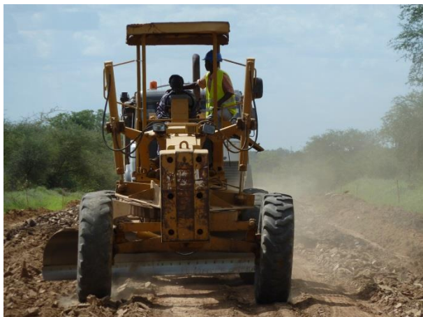
Figure 4.1 – Motor grader used for maintenance of unpaved rural roads, (Image: Intech Associates)
