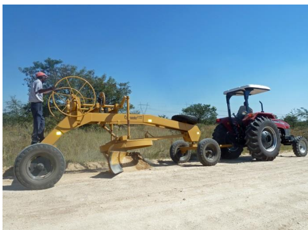
Figure 4.3 – 2 tonne towed grader manufactured in Zimbabwe for more than 50 years (Image: Intech Associates).
