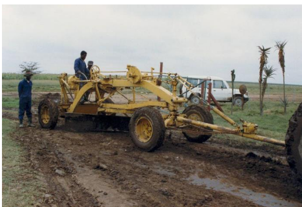
Figure 4.4 – Pre-war Caterpillar tractor towed grader with rubber tyre modifications. Still in regular use after 50 years (Image: Intech Associates)
