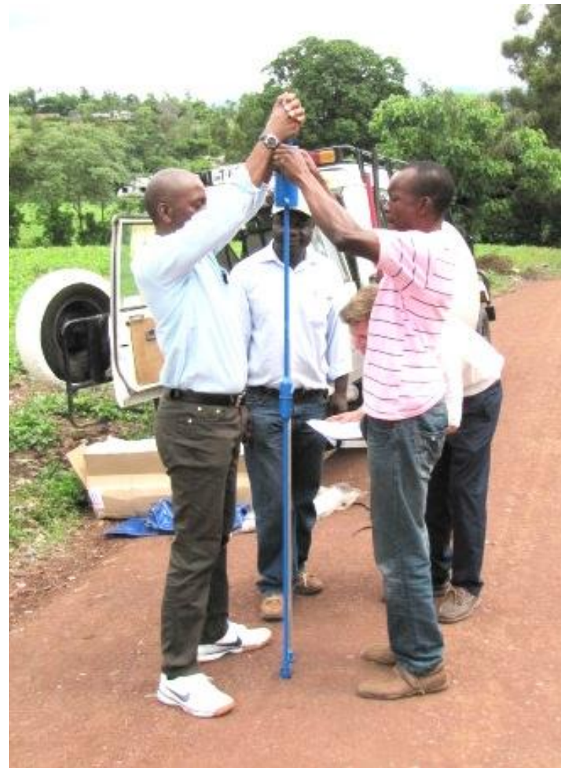
DCP test in process
