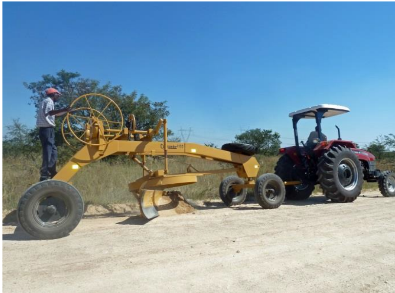
Photo 1 Two tonne tractor-towed grader manufactured in Zimbabwe (Photo: Rob Petts)
