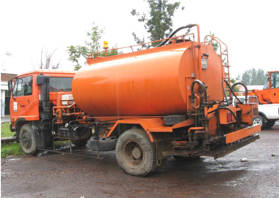
Figure 2 Second Bitumen distributor now in disrepair
