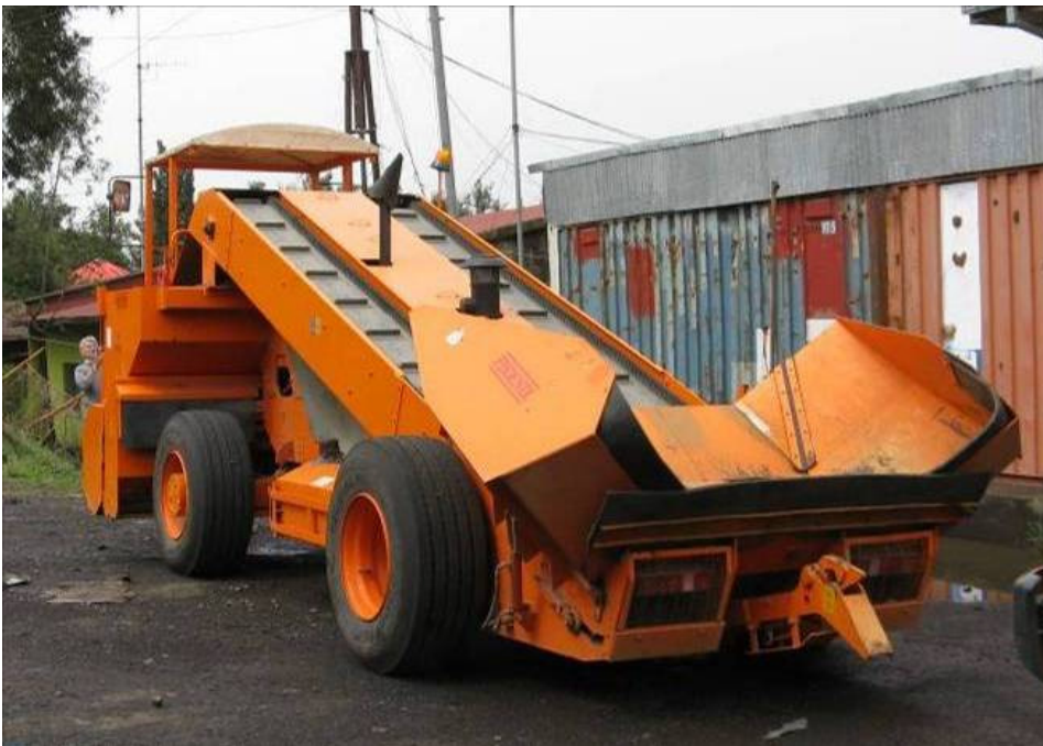
Figure 4 Self propelled chip spreader used in February 2012
