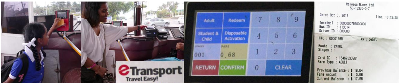
Figure 12 Montage showing bus e-ticketing in Fiji, with tap in, ticket collection, driver's panel and sample ticket
