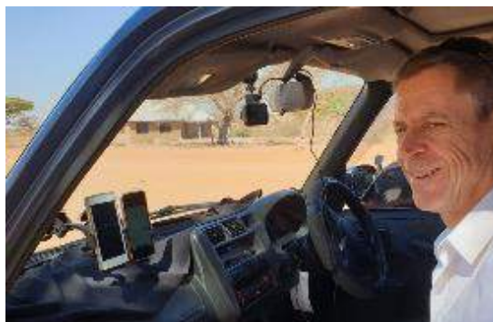
Figure 2 Vehicle set up for drive-through survey with DashCam and smart phones with apps
