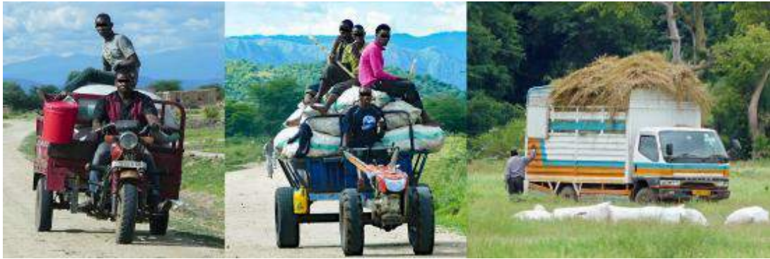
Figure 9 Motorcycle three-wheeler or 'toyo' (left), 2-wheel tractor (centre) and light truck (right)
