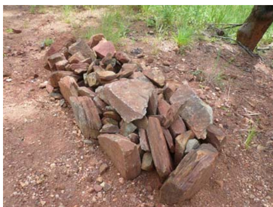
Rejected stones – some laminar, some non-laminar
