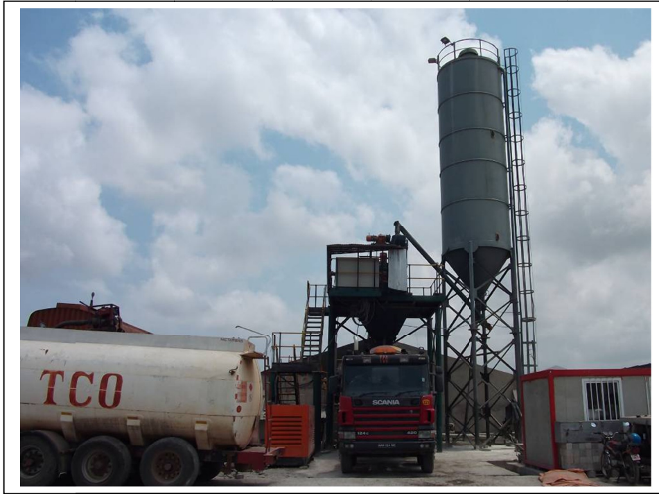
Figure 4-1 TCO's Concrete Plant for ETB Mixing
