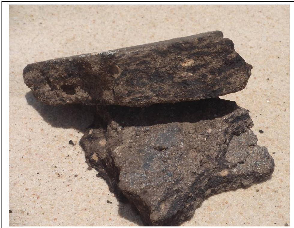
Figure 4-4 Block of cured ETB from trial section
