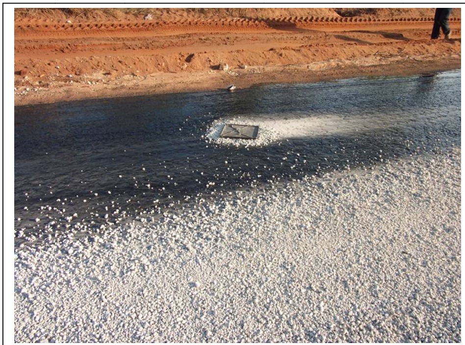
Figure 4-7 Tray test for control aggregate application rate
