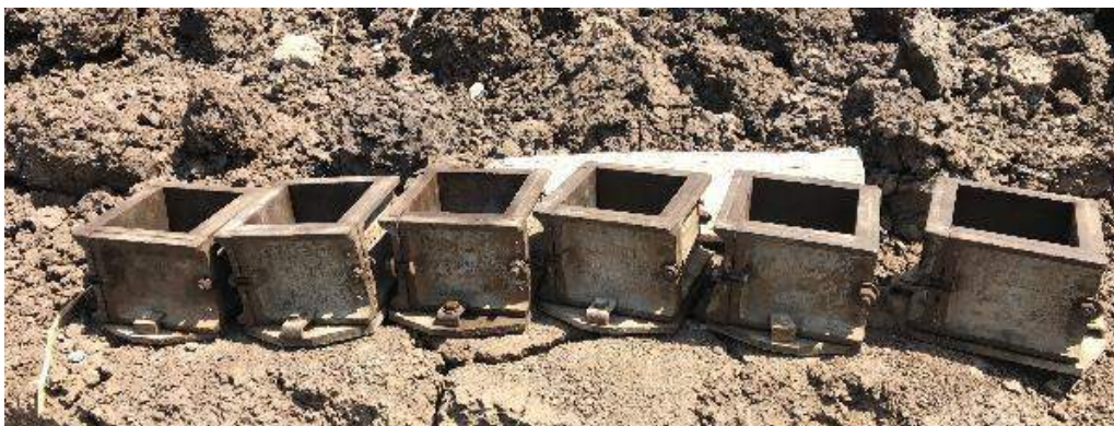
Figure 1.8 Mould for concrete compressive strength test specimens
