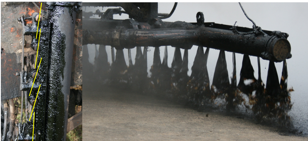
Photograph 3 Flair interference due to wrong angle settings
